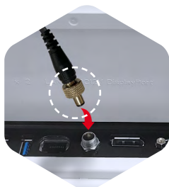
Tighten connection for power
